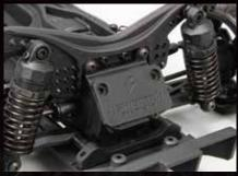
While the previous model mounted the ESC near the chassis center, a new 3D-printed plate-shaped mount is included. You can choose the mounting position above the differential case or on the rear overhang. Adjusting the weight distribution enhances the feel of carving corners and improves stability during high-speed turns.
