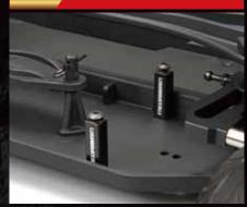
A vertically mounted servo mount is included. This makes it easier to align the transmitter's EPA settings between left and right channels, creating an environment where the steering gyro's performance can be maximized.
